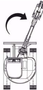
3 - pressing the pedal to the RH side swings the digger boom to the RH side.
