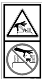
Fig. 52: Hydraulikoliebeholder under tryk
